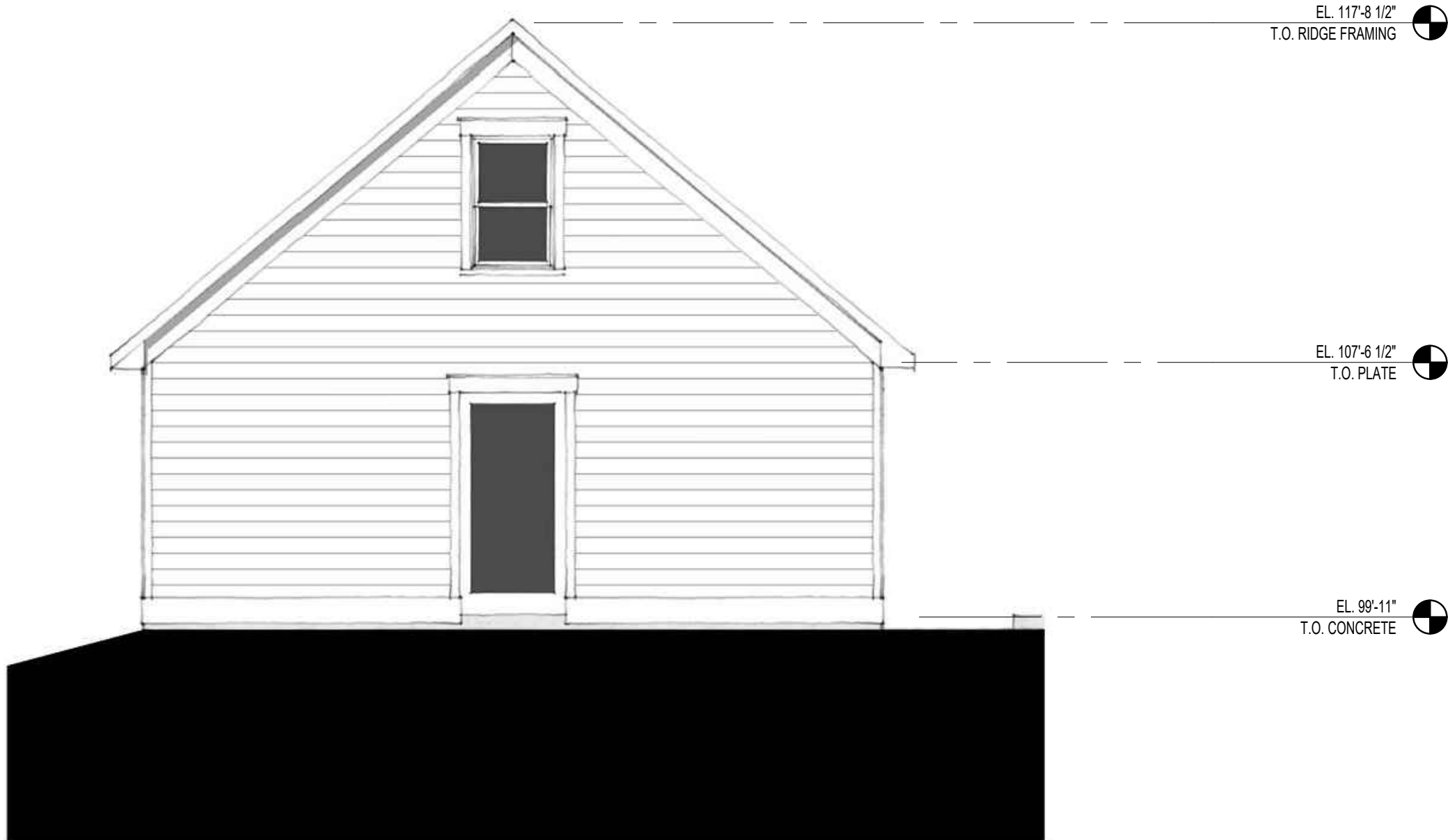
2 GARAGE WEST ELEVATION A2.3 SCALE: 1/4" = 1'-0"
