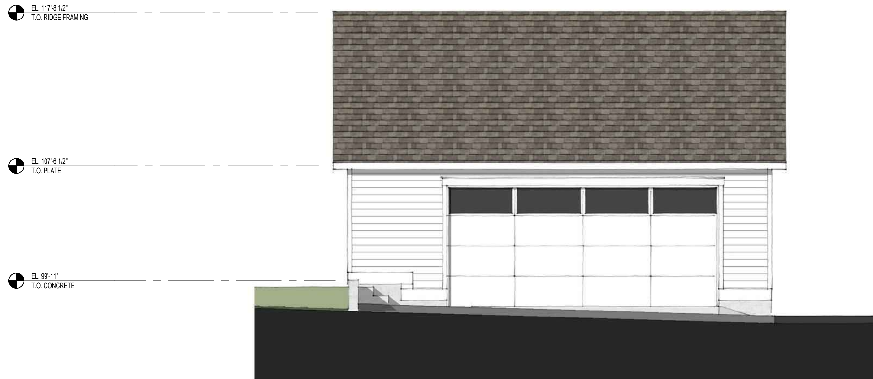
1 GARAGE SOUTH ELEVATION A2.3 SCALE: 1/4" = 1'-0"
