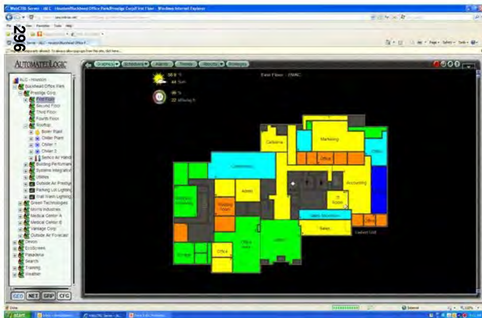
Automated Logic "Environmental Index" Thermograph Screen-Shot
