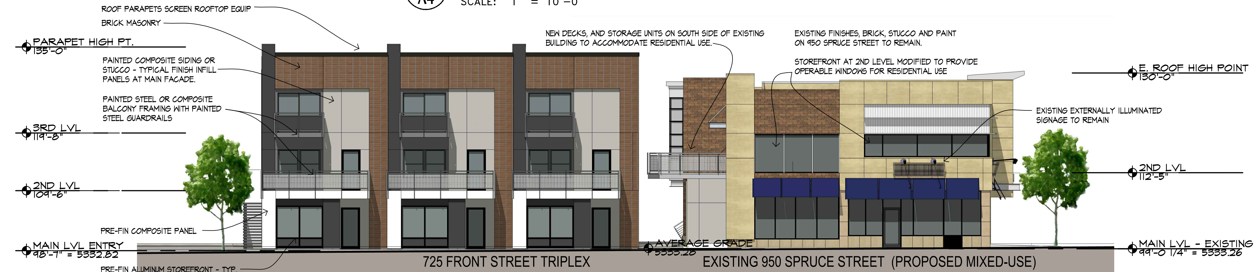
C1 A4 EAST ELEVATION – FRONT STREET SCALE: 1" = 10'-0"
