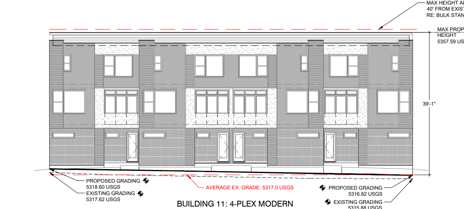
BUILDING 11 - SOUTH ELEVATION
