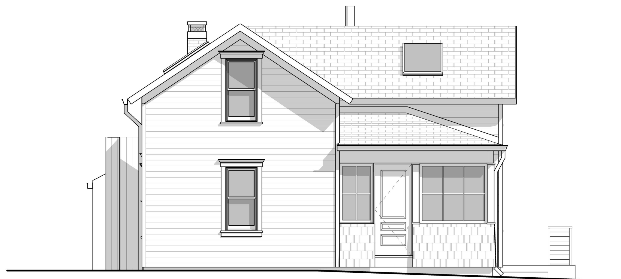
2 A.3 1/4" = 1'-0" NEW WEST ELEVATION
