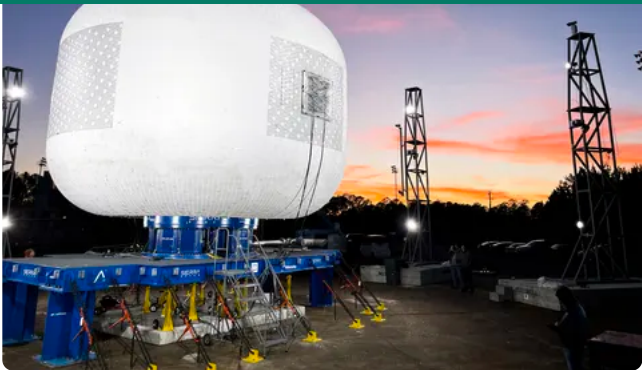
Sierra Space's second full-scale test next month will be another Ultimate Burst Pressure (UBP) test to validate the technology's ability to perform flawlessly in the unforgiving conditions of space. (Photo: Sierra Space)
