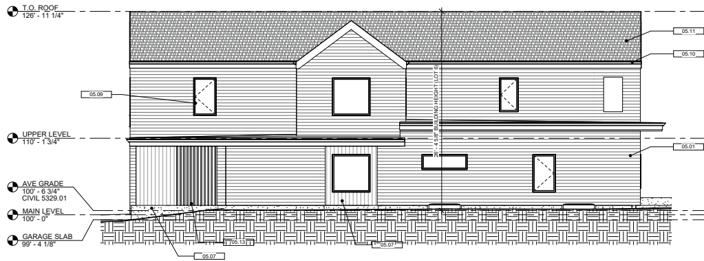
② SDP - EAST ELEVATION (REFERENCE LOT 4) 3/16" = 1'-0"
