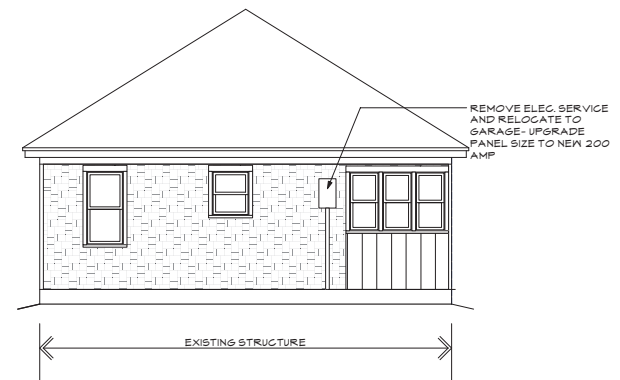
EXISTING WEST ELEVATION 1/4" = 1'0"
