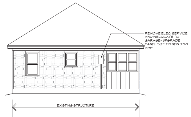
EXISTING WEST ELEVATION 1/4" = 1'0"
