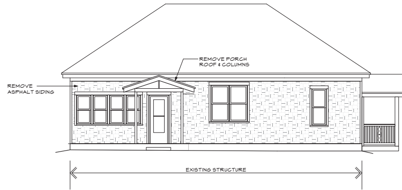
EXISTING SOUTH ELEVATION 1/4" = 1'0"
