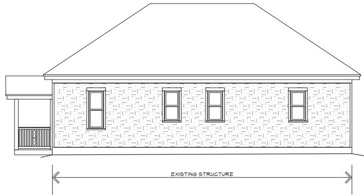
EXISTING NORTH ELEVATION 1/4" = 1'0"
