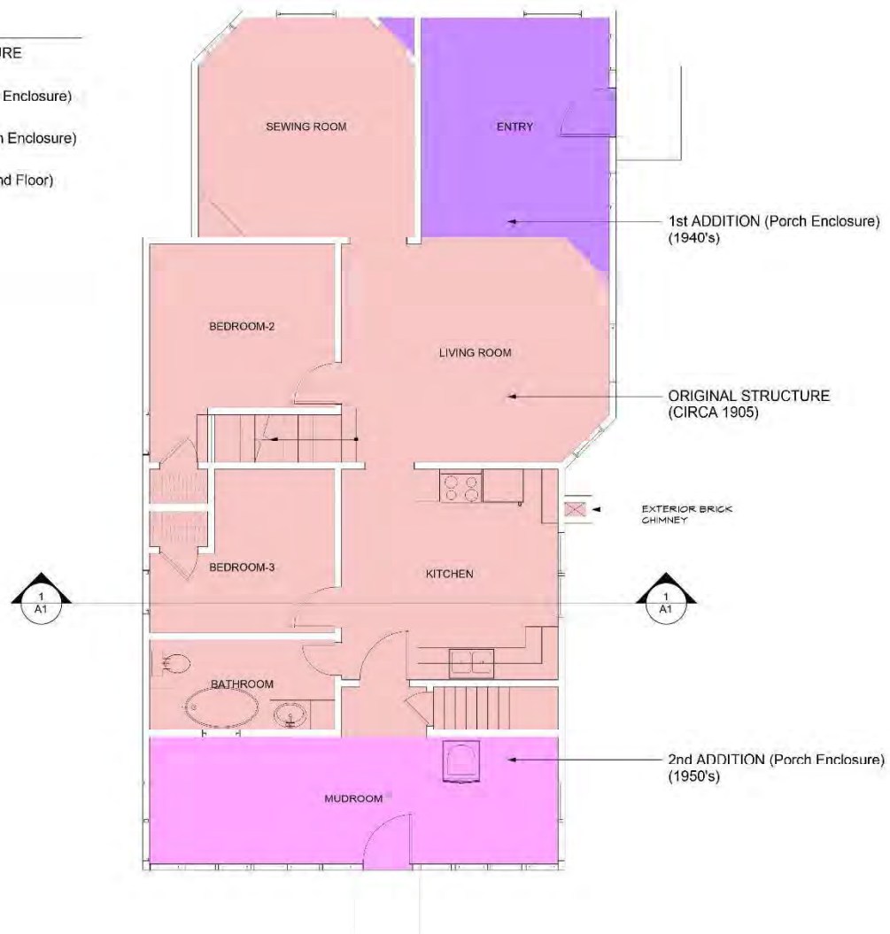
Building Construction History Plan- First Floor
