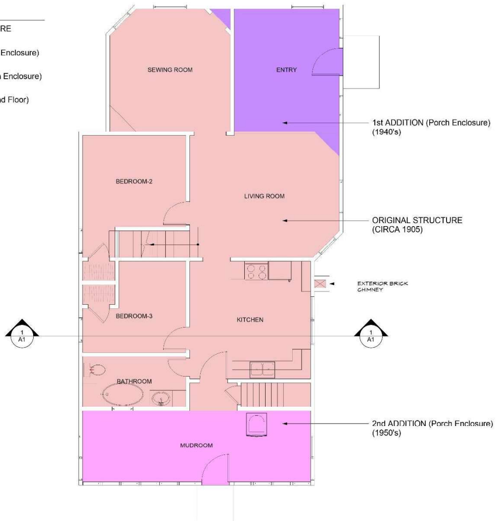
Building Construction History Plan- First Floor
