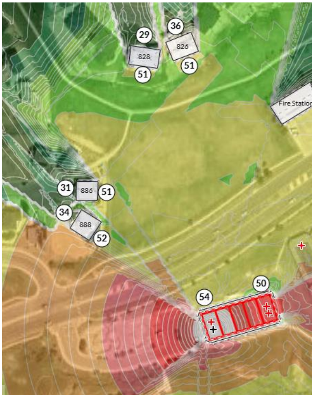
Figure 15a – Source 2, 18 ft absorbing barrier on N wall and 10 ft absorbing barrier on S wall
