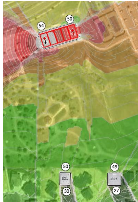
Figure 15b – Source 2, 18 ft absorbing barrier on N wall and 10 ft absorbing barrier on S wall
