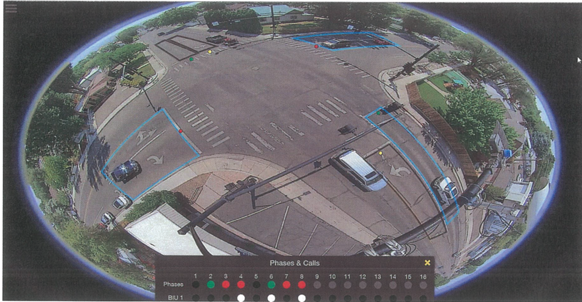
Example of a Basic single camera Gridsmart intersection setup
