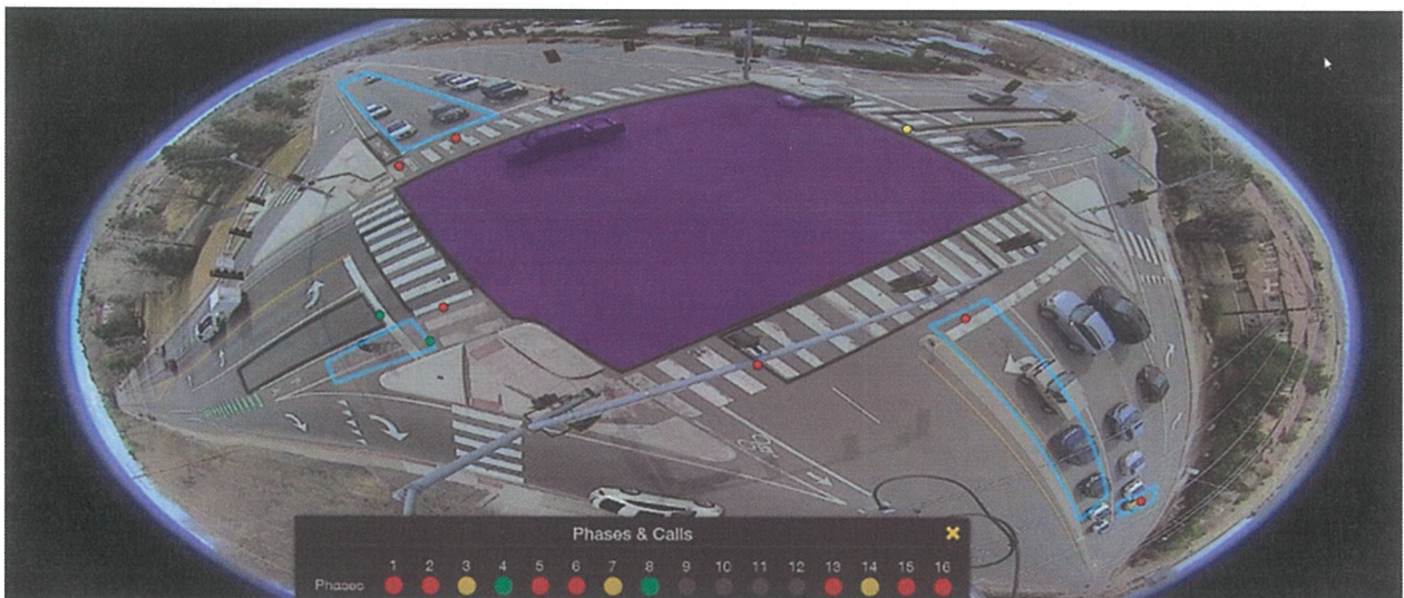
Example of a Gridsmart operating with Bike lane and Bike Box Differentiation
