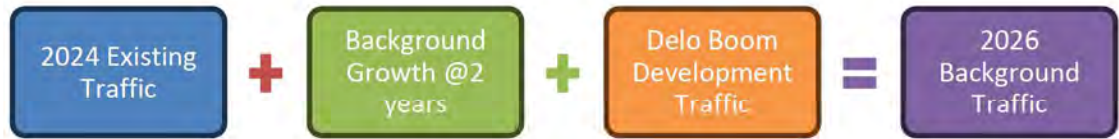
Figure 3: 2026 Background Schematic Diagram
