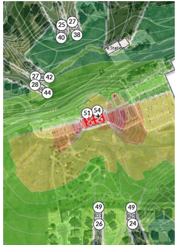
Figure 21c – Source 3, 16 ft/10 ft absorbing barrier Figure 21d – Source 4, 16 ft/10 ft absorbing barrier
