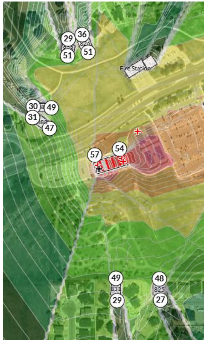
Figure 17a – Source 2, 16 ft absorbing barrier on north court side, 16 foot reflecting barrier on west court side (transparent), 10 ft sound absorbing barrier on south court side
